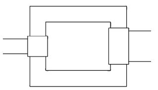
A transformer is made up of a primary coil from the alternating current (ac) input, a secondary coil leading to the ac output and an iron core. A transformer has one coil of insulated wire on each side. There are a greater number of turns of wire on the primary coil than there are on the secondary coil.
